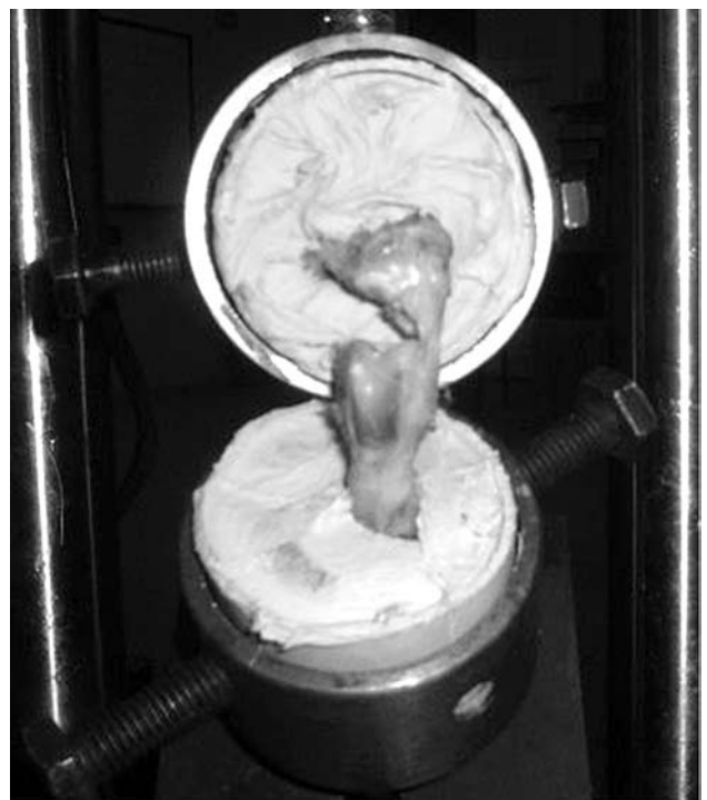
Figure 2. Specimens are mounted to the universal testing machine.
