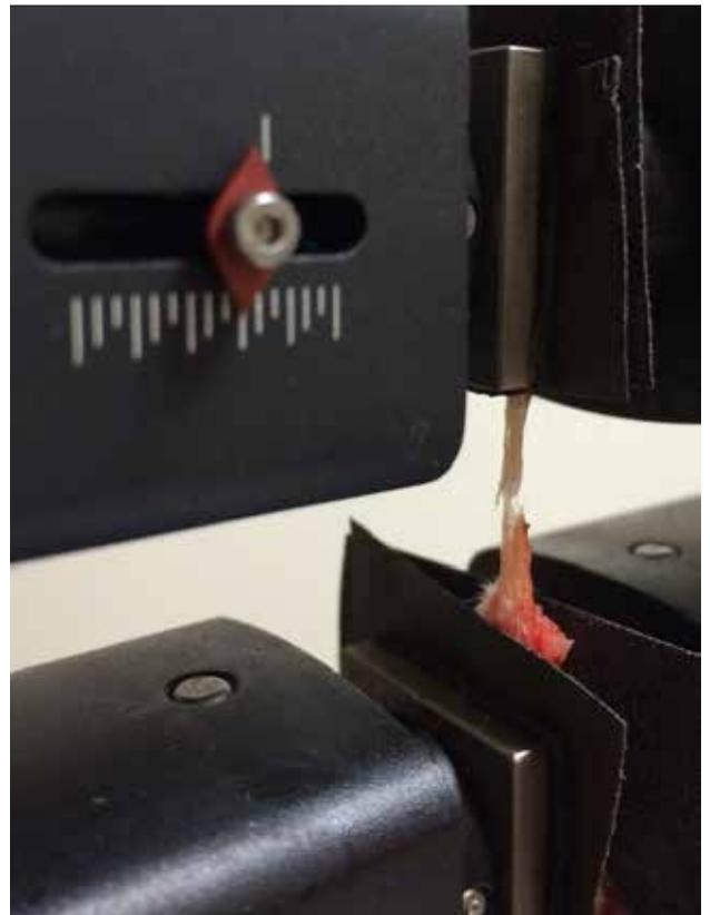
**Fig. 4.** Biomechanical analysis of the Achilles tendon; tendon visibly ruptured at the mid-zone. [Color figures can be viewed in the online issue, which is available at [www.aott.org.tr](http://www.aott.org.tr)]
