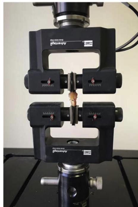
Fig. 2. Placement of the repaired meniscus on the biomechanical tester.
