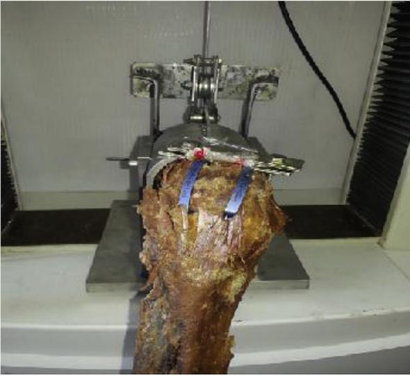
**Fig. 4.** All samples were tested by exerting a knee motion from 90° flexion to full extension by applying traction to the quadriceps tendon through a steel-sling.
