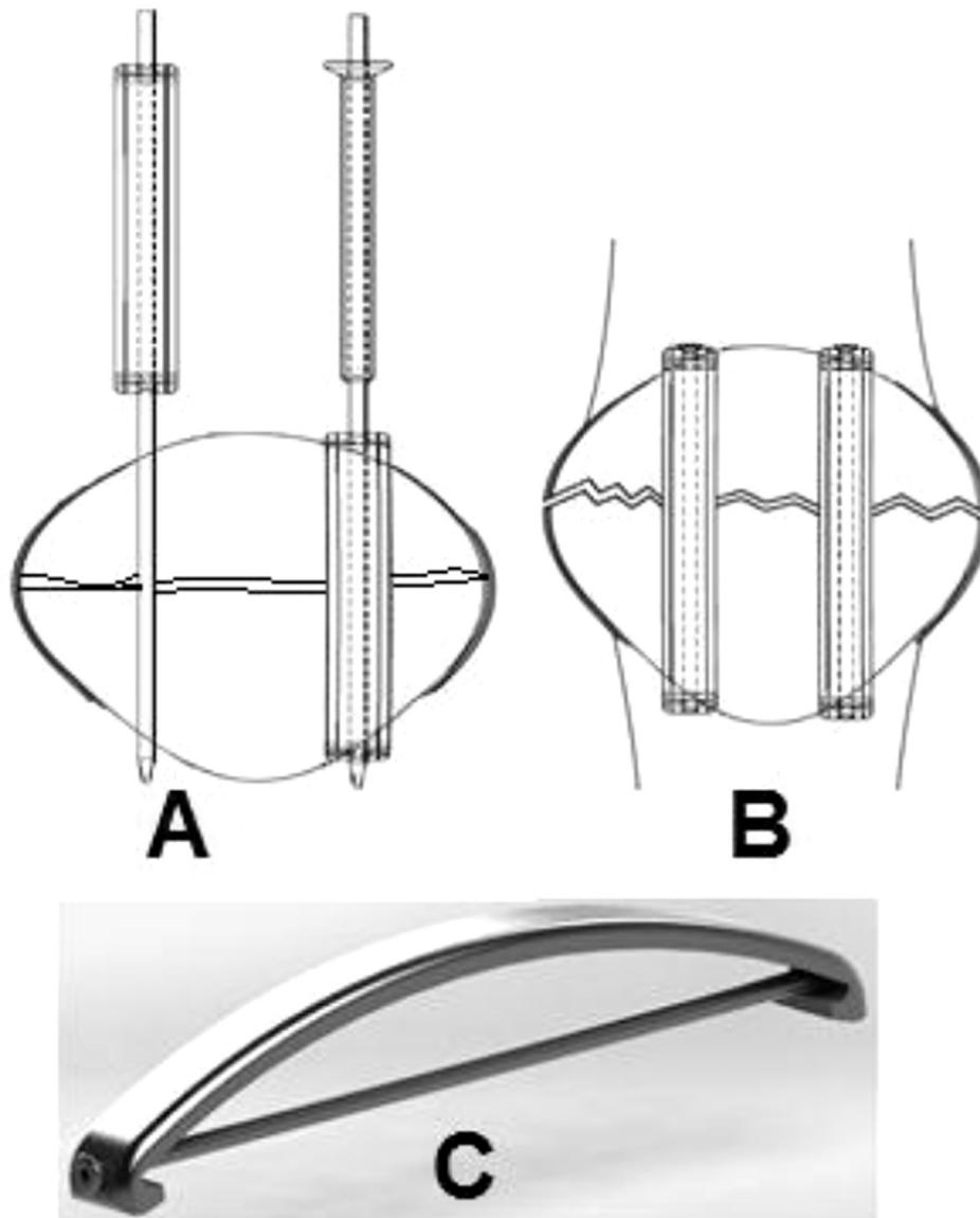
**Fig. 2.** The technique of anatomical plate application, (A) K-wire insertion after anatomical reduction, (B) Replacement of the anatomical patellar plate through the K-wires, then placement of the cannulated cortical screw through the K-wire. (C) The anatomical patellar plate.
