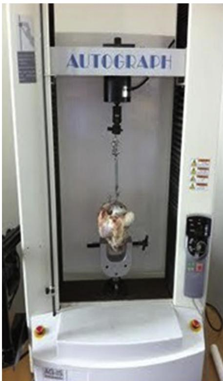
Fig. 5. Pull-out test was used to determine the load (N)—displacement (mm) curves at rate of 20 mm/min with computer-assisted Shimadzu Autograph AGS-X 10 Kn universal testing machine (Shimadzu Corp., Kyoto, Japan).
